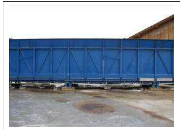
Figure 7 – Solids feeding unit which introduced feedstock into the primary digester via a screw thread
