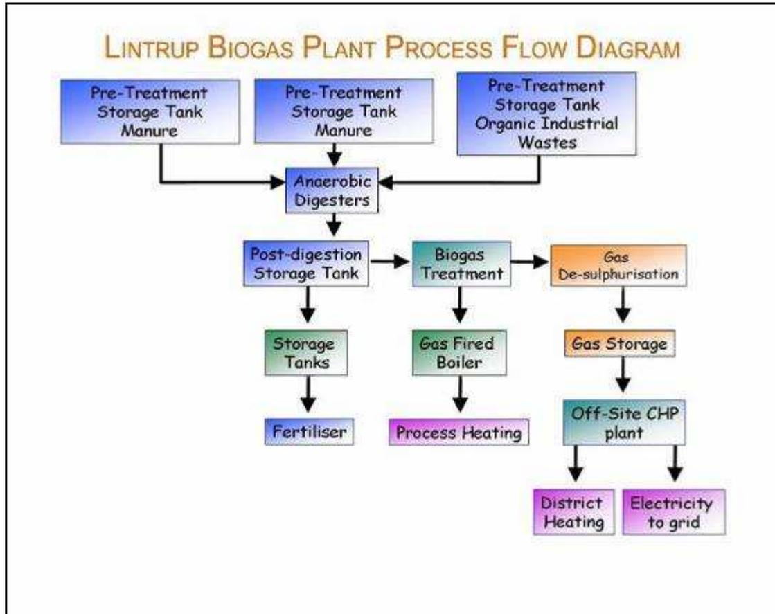
**Figure 1 Lintrup Biogas Plant process flow diagram**
