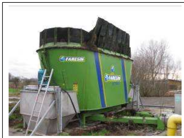
Figure 5 – Double end solids feeding unit with screw thread feeds to Digesters 1 and 2
