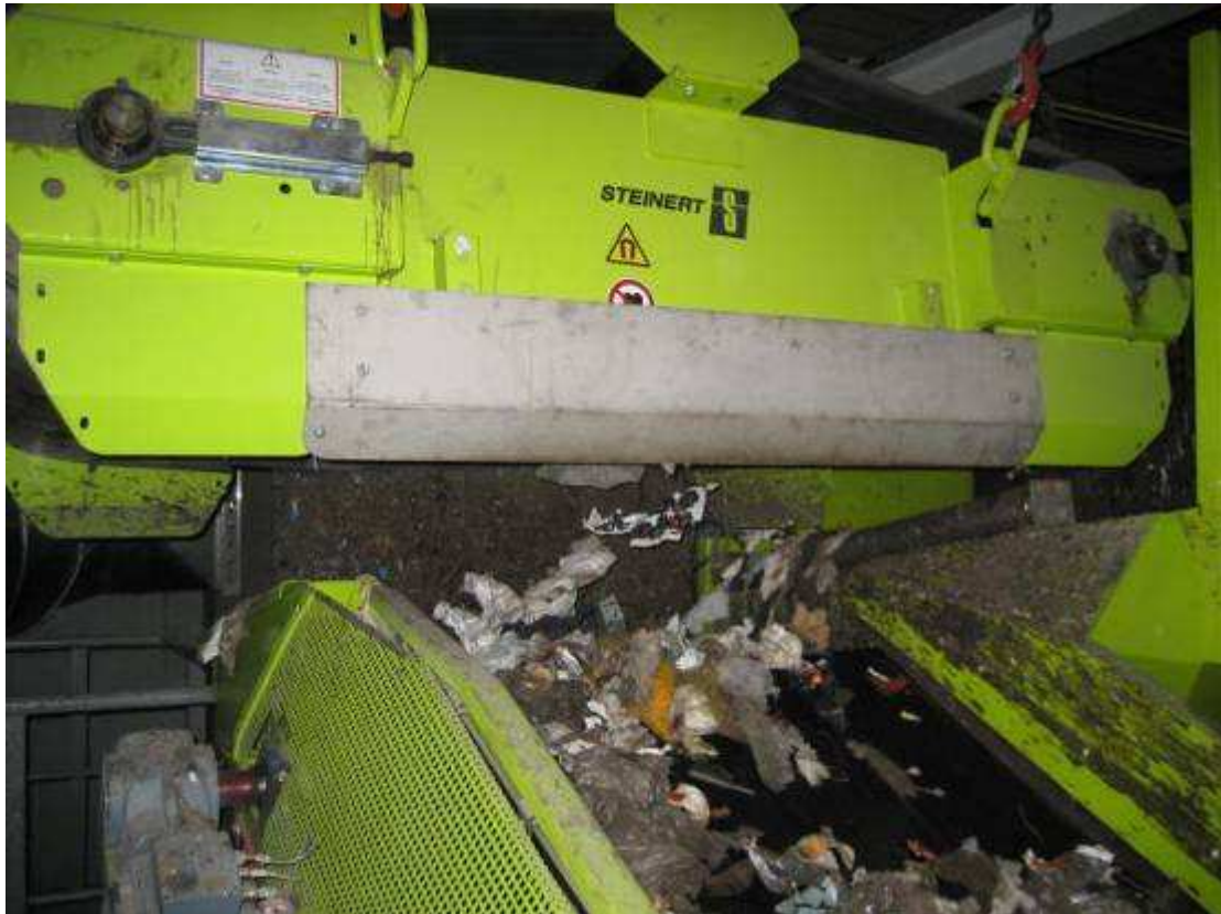
Figure 7 ‘Light fraction’ separation by wind sifting
