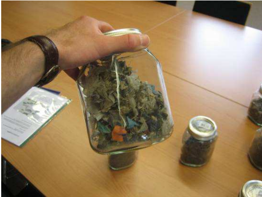
Figure 10 RDF from residual waste stream
