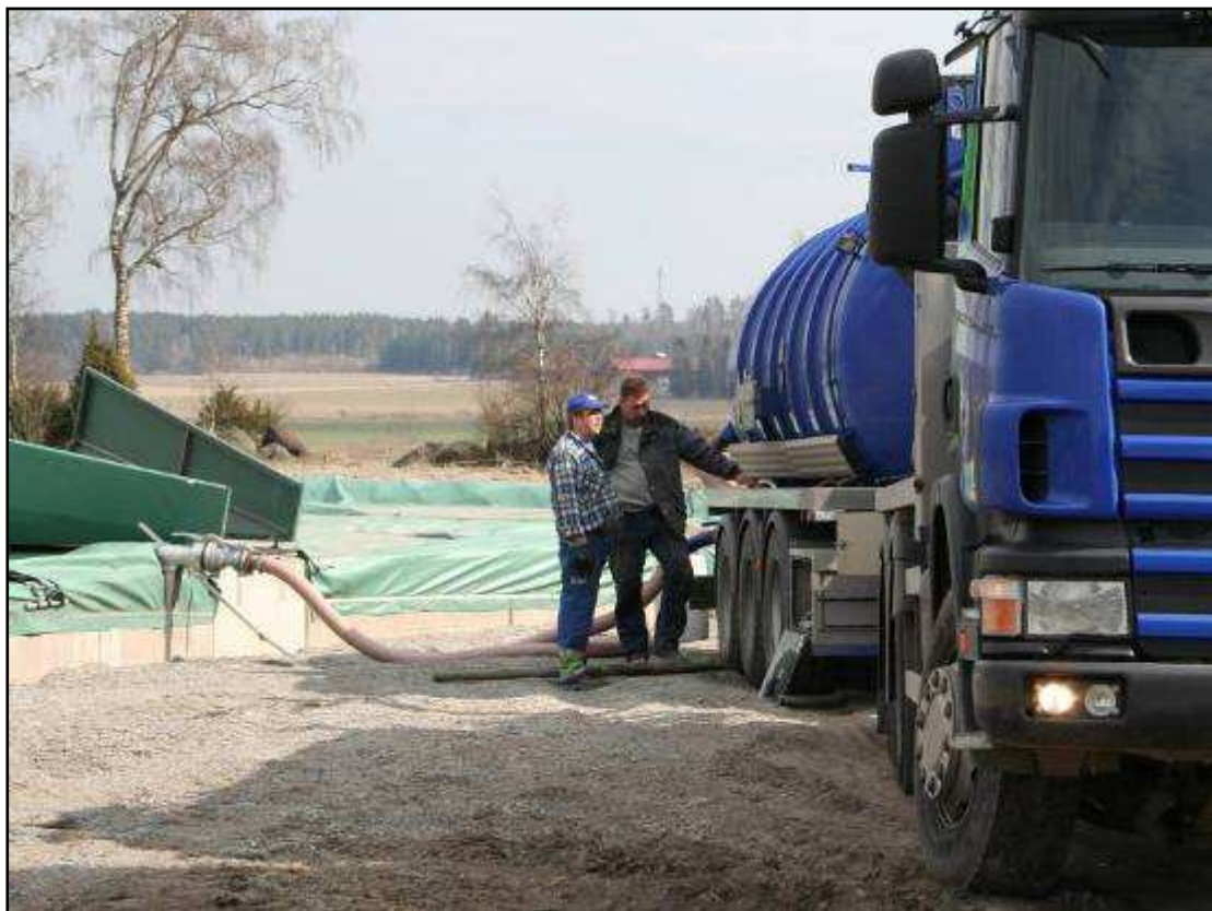
Figure 21 Liquid digestate transport to storage tanks (Pettersson, 2006)
