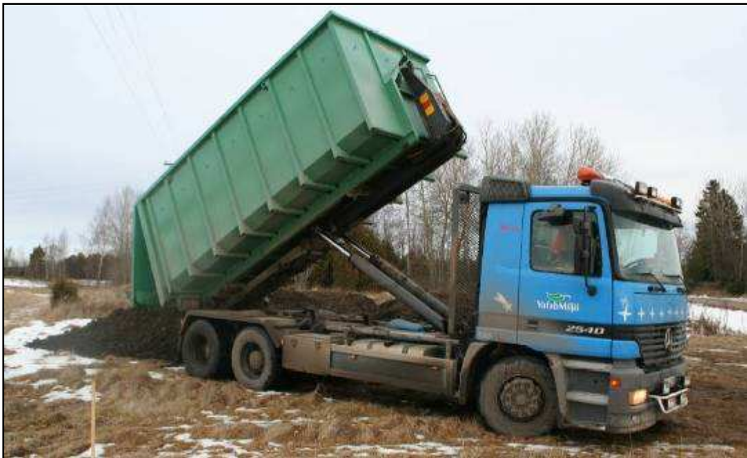
Figure 26 Truck unloading solid digestate container on farmland (Pettersson, 2006)
