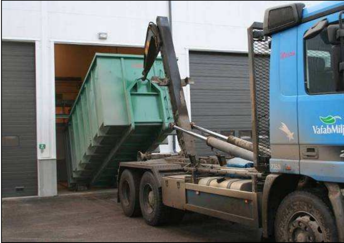
Figure 25 Truck removing solid digestate container from plant (Pettersson, 2006)
