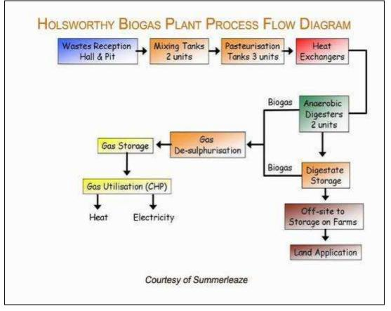
Figure 1 Process flow diagram of Holsworthy Biogas Plant
