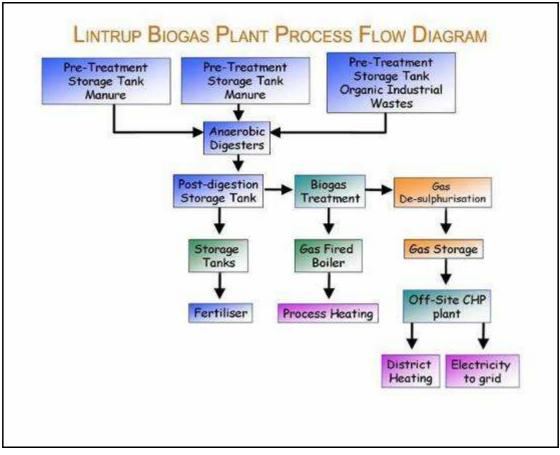
Figure 1Lintrup Biogas Plant process flow diagram
