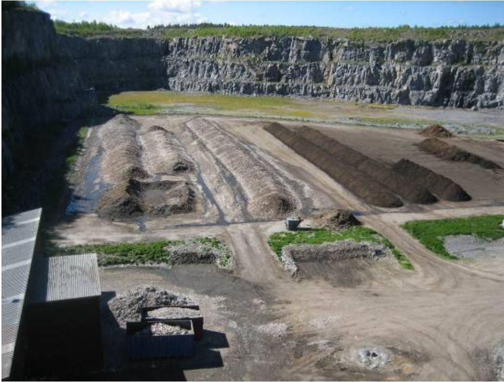
Figure 149 Windrow composting of unsorted MSW and digestate at Stormossen
