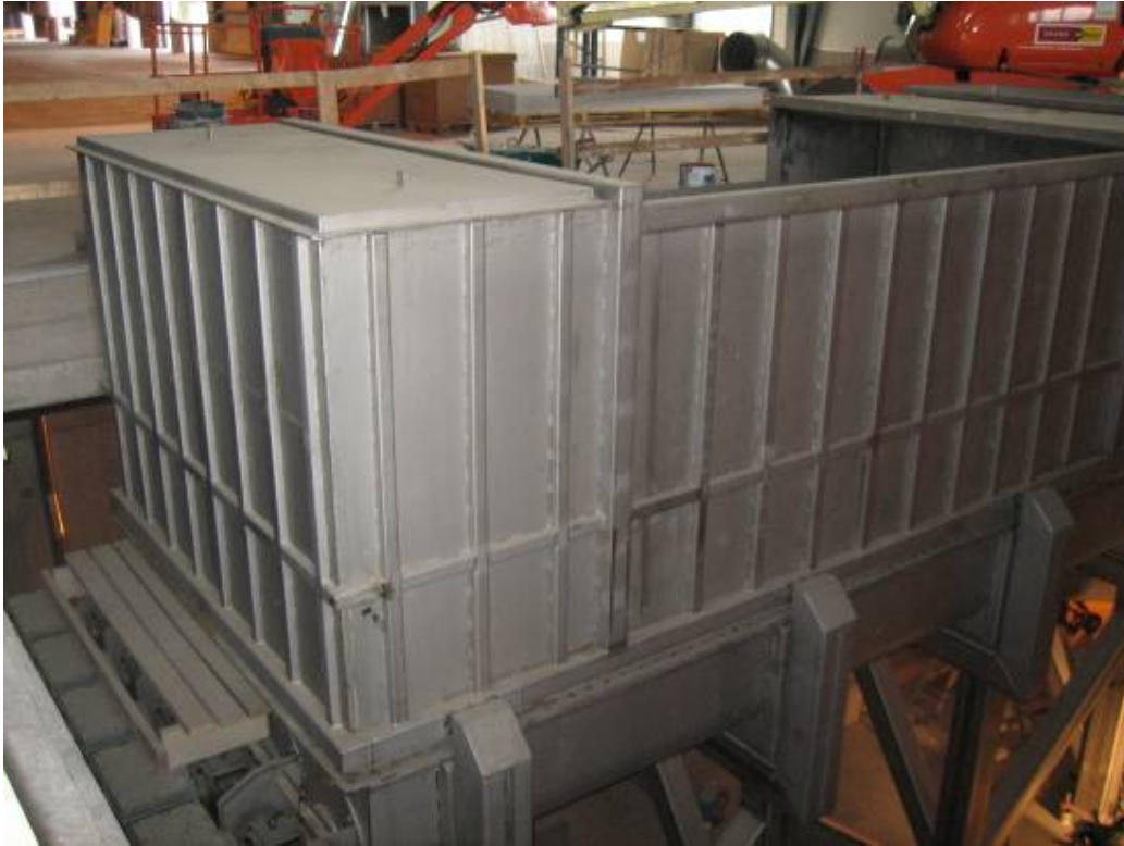
Figure 68 Wastes reception pit at Torsvik
