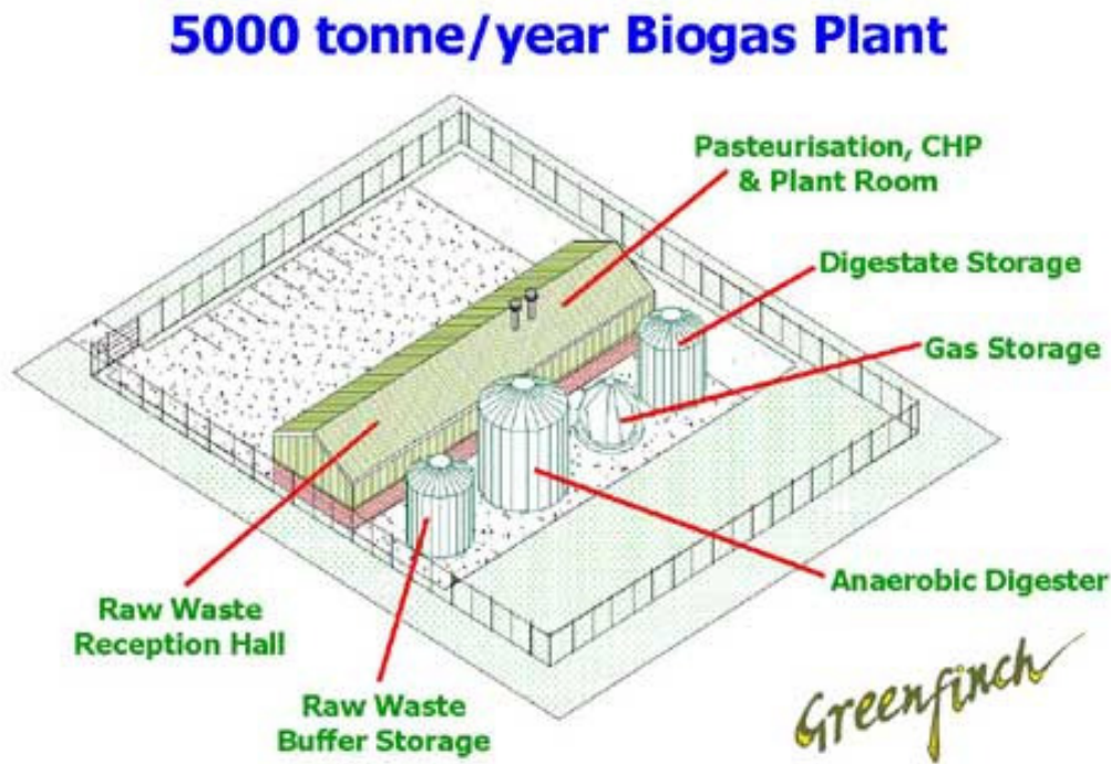
Figure 78 Illustration of aerial view of Ludlow Biowastes Treatment Plant (Greenfinch website, accessed April 2006)
