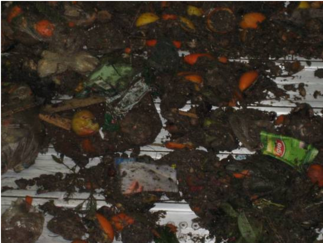
Figure 120 Municipal biowaste as delivered to wastes reception pit
