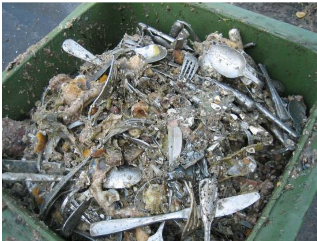
Figure 89 Metals removed from food wastes
