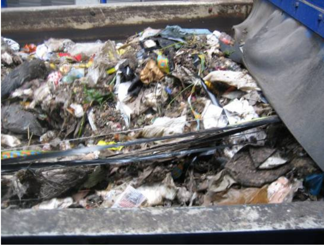
Figure 197 Cassettes, rope and other wastes becoming tangled in moving parts of process
