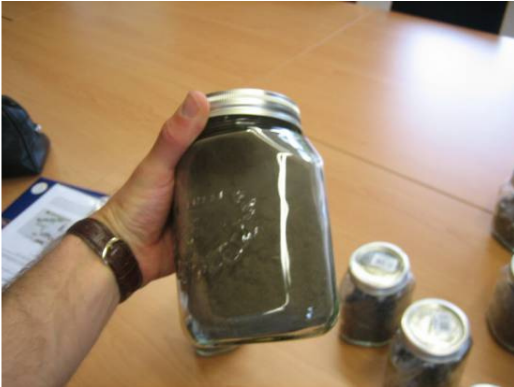
Figure 256 Fine grade SRF from residual waste
