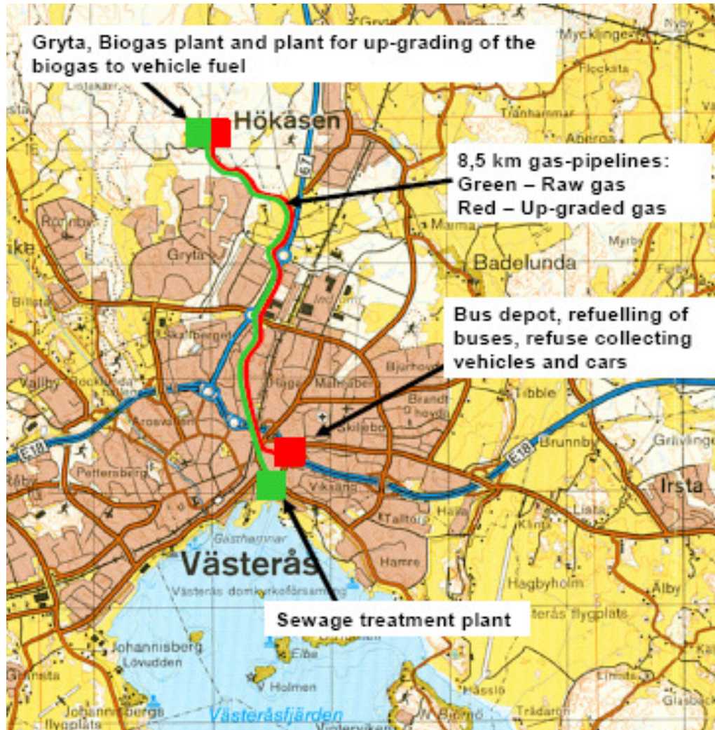
Figure 154 Location of the production sites for biogas and filling stations for vehicles in Västerås (Agropti Gas Promotional Information)
