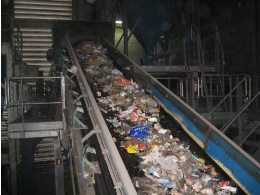
Figure 220 Waste stream from first trommel sieve to shredder
