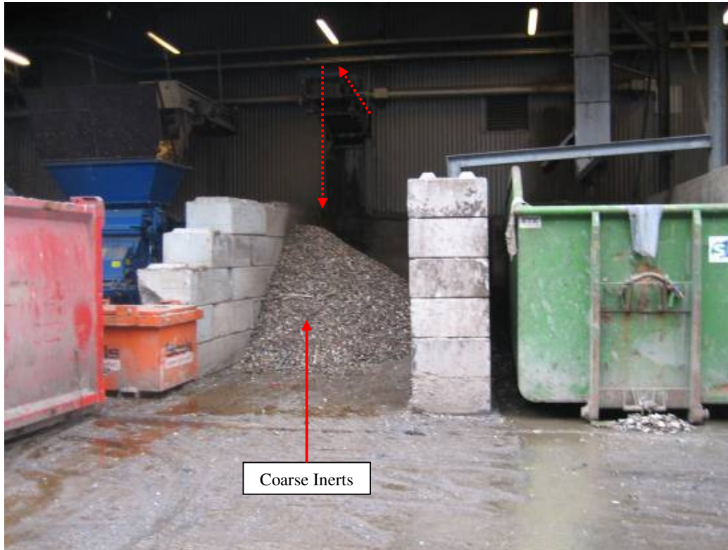
Figure 212 Coarse inerts removed from organic waste stream
