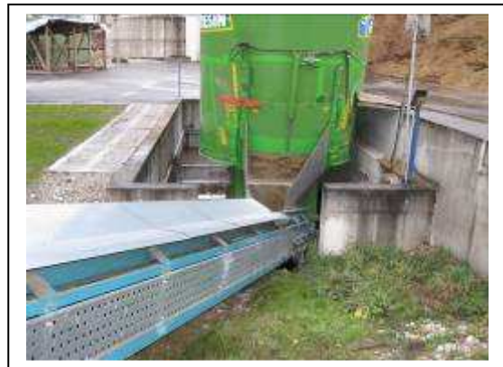
Figure 16 – Solids feeder discharging silage to conveyer
